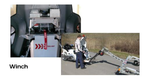
The winch on the rear of the Retriever will allow for the operator to partially load and unload the towing unit on to/from the motorcycle automatically. This will not only help in preserving the energy of the operator, it also improves the safety whilst operating. Another great benefit would be that the winch can be used to load a car on to the towing unit.
